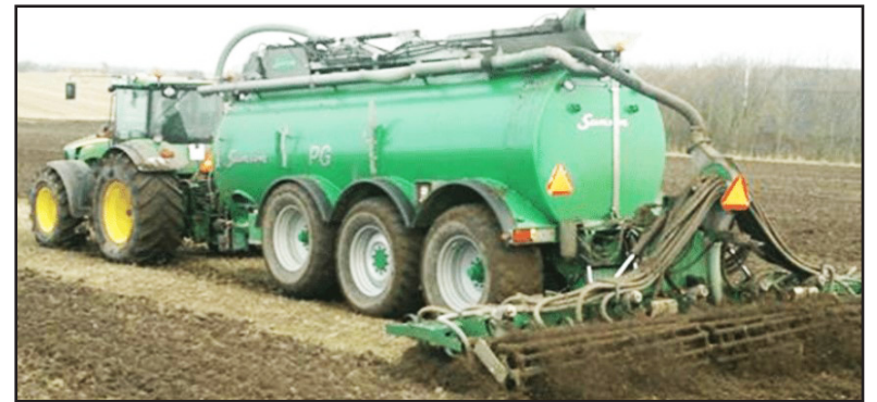
Subsurface injection of raw slurry using a slurry tank, tiller and nozzles. Photo credit researchgate.net, Leaching of Elements from Soil in Grassland Field Crops Treated with Raw and Acidified Slurry.
